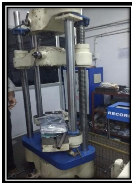
PLATE 4 Tensile tester used for composites
