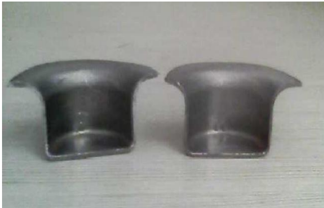
FIGURE 12: CUT PIECES OF DRAWN COMPONENT
