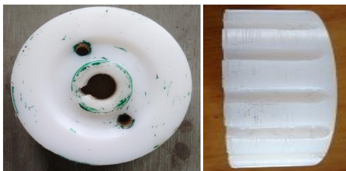
Fig. 2 A view of seed metering device fabricated in laboratory (Plate type ) for sowing soyabean seeds.
