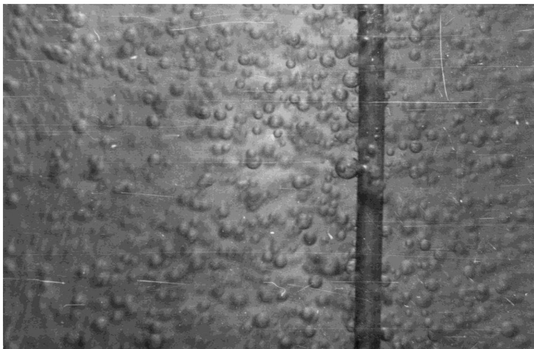
Fig. 2. To determine the size of the dispersed phase droplets
