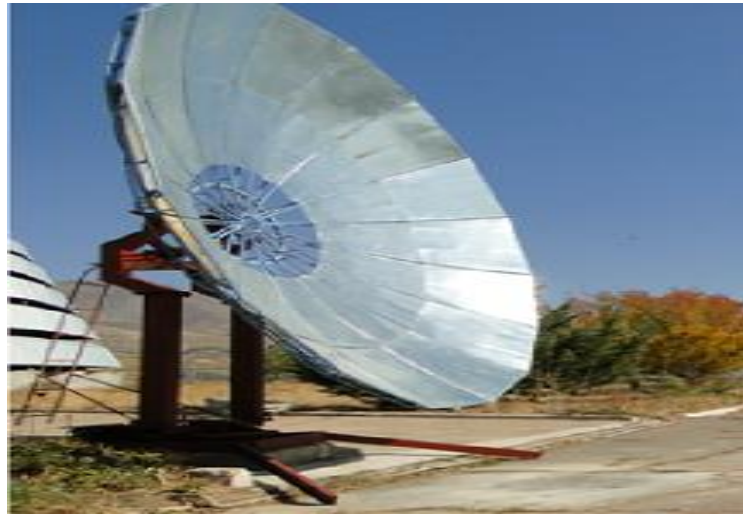
Fig. 7. General view of an autonomous concentrator with a diameter of 6.3 m
