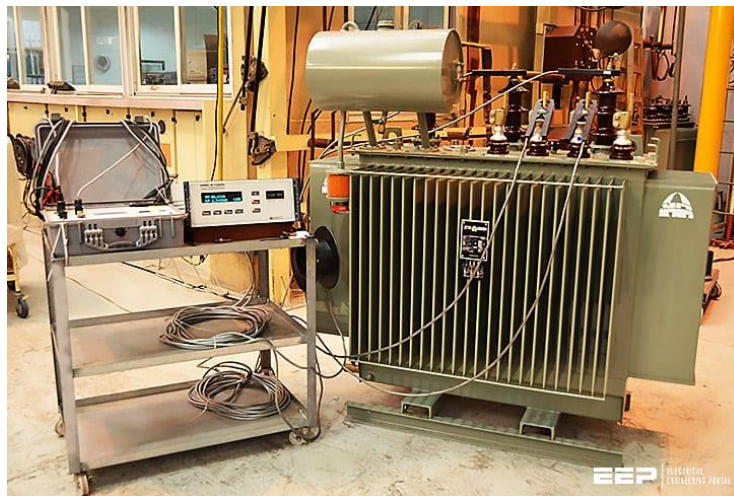
Figure 4: No- load losses of the transformer [electrical-engineering-portal].
